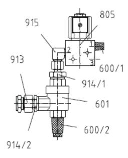
Connection 1 = Ventilation Connection 2 = Drive Connection 3 = Control air
